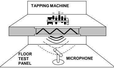
Figure 1: IMPACT NOISE TESTING FACILITY
