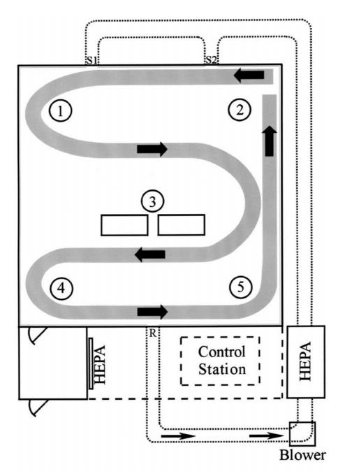
*Figure 1.* Diagram of the experimental room. The shaded area represents the walking path for trials on contaminated flooring materials. The room air handling system delivers HEPA-filtered air into the room through 2 supply registers (S1 and S2) and exits through one return register (R). Sampling stands (locations 1-5) support temperature and relative humidity probes. Air samplers were located in the center of the room (rectangular boxes).
